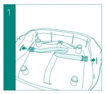
With the upper seat upside down, pass the ends of the securing strap through the slots at the sides as shown.
