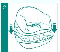
Place the upper seat onto the base as shown, and press down firmly to engage the clips at the sides of the seat (see diagram 3).
