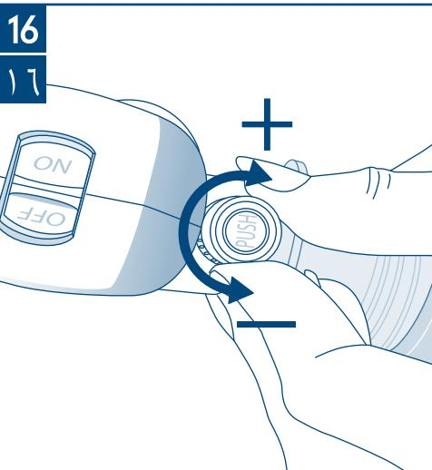
**The suction regulator can adjust the suction level when pumping**
