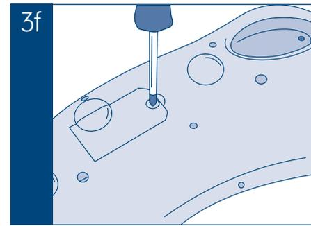
The Light and Sound Keyboard takes 2x AA batteries. Unscrew the battery door using a Phillips screwdriver and insert batteries (dia 3f).
