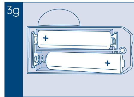
Ensure battery polarities are correctly aligned with the polarities within the battery compartment (dia 3g).
