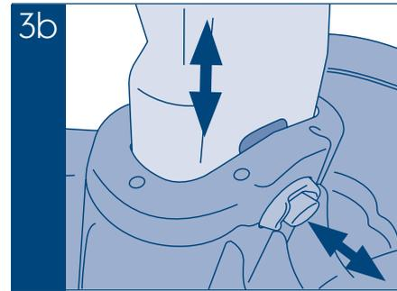
The height of the Activity Station can be adjusted by pulling the red button and sliding the leg up or down, releasing the button to lock into the available slot (dia 3b).
