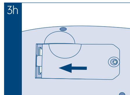
Replace the battery door, slide into place and tighten screw to secure (dia 3h).
