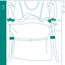
The bag is attached by four straps and buttons. Two fix above the hinges and two fix on the back legs as shown.
