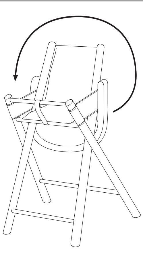
Your Folding Highchair is supplied fully assembled and ready for use. After removing all packing material, the highchair may be opened and the tray swung over the back of the high chair to rest on the front crossbar. Ensure that the clips are in line with the crossbar, press down firmly on the tray to engage both locks. Do not use the highchair without ensuring that the tray is locked in position.
