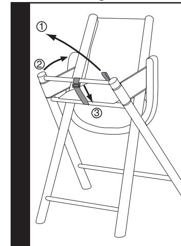
Stand in front of the highchair, release the tray clips by lifting both tabs and swing the tray over and behind the chair. Locate the fabric tab (1) at the join between the seat back and seat base.
