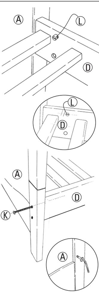
When assembling as a cot only use one barrel nut (L) on each corner of base (D). ALWAYS USE THE TOP HOLE IN THE COT BASE.
