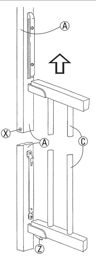
Ensuring that the "PUSH" label faces outwards, locate all four drop side slides onto the runners. Gently pull lower spring clips (Z) outwards and raise side into the closed position. It will engage automatically.
