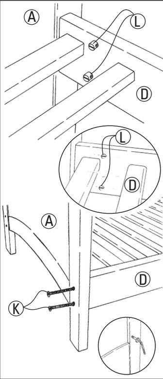
When assembling as a bed use two barrel nuts (L) on each corner of base (D)
