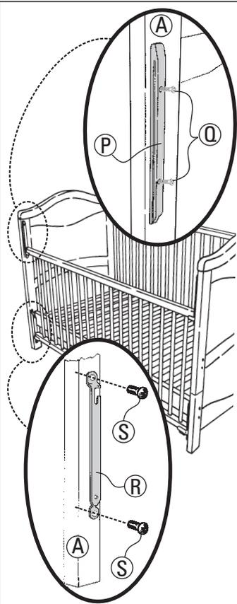
Attach the four drop side runners to the cot ends (A). To ensure that they are positioned correctly, align holes in runners with holes in cot ends.
