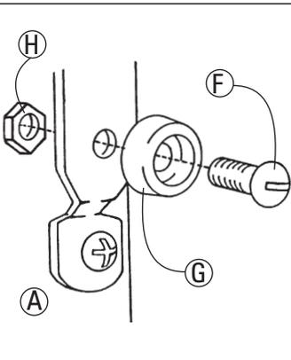
Attach the two rubber stops (G) to the lower metal runners using bolts (F) and nuts (H).
