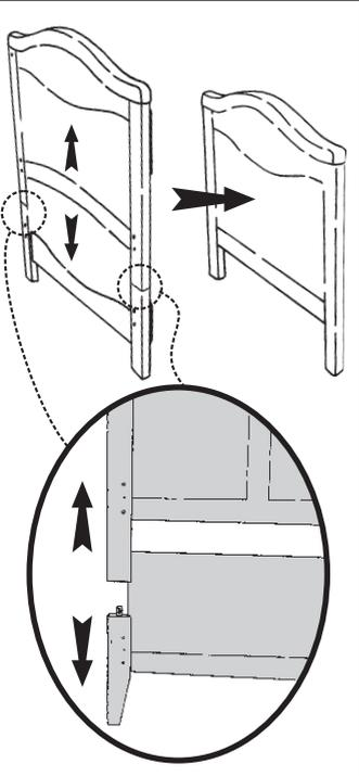
To convert the cot to a bed, first remove the two sides and four drop side runners, then detach the cot ends.
