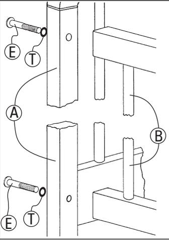
Use four bolts (E) with protective washers (T) to attach fixed side (B) to cot ends (A). Do not fully tighten fittings at this stage.
