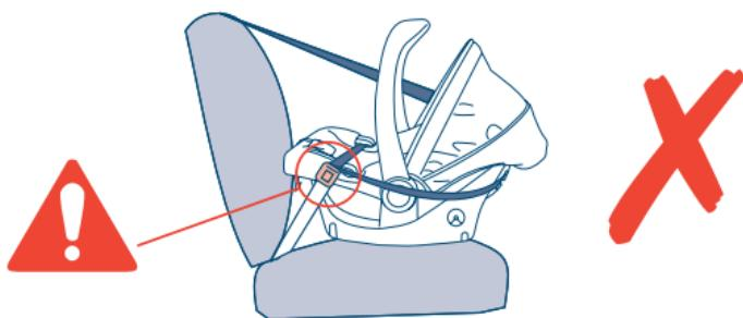
This child restraint must not be used if the adult safety belt buckle is positioned as shown. If in doubt please contact Mothercare. Contact details are given at the end of this guide.
