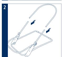
Place the frame on the floor with the open tubes pointing upwards.
