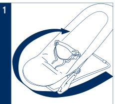
The cradle can be folded for storage. First remove the toy bar, then pull the base around to rest against the seat cover.
