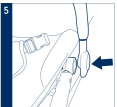
Locate the ends of the toybar over the sockets on the side mouldings.
