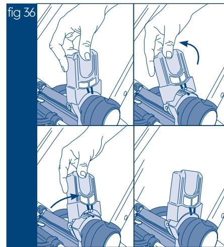
Adjust the adaptors on the chassis frame. push each adaptor inwards then backwards into its new position, ensure that the indicators on the adaptors line up with the infant carrier image. Compatible infant carrier is the Maxi-Cosi Cabriofix.
