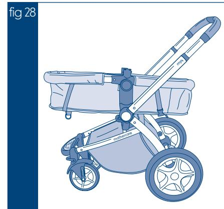
With the pushchair in pram mode, undo the four harness clips and move these to the edge of the pram unit. Remove the hood and bumper bar.
