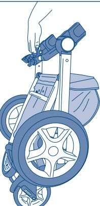
Ensure the folding catch is engaged, then use the handle in the centre of the chassis frame to carry the unit.
