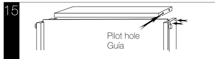
Attach the backs using 4 domed screws (35mm) for each drawer. Do not over tighten.
