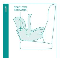
Your car seat is fitted with a seat level indicator. This is designed to help you ensure that the seat is positioned at the correct angle.
