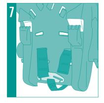
**Step 4** Re-attach the loops on the shoulder straps to the slots on the metal plate. Check that the loops are within the metal plate slots and are securely attached.
