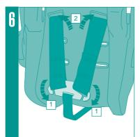
Before you begin loosen the harness straps using the 'one-pull' adjuster as described on page 11.
