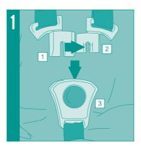
The buckle is fastened by locating parts (1) and (2) together then pushing into the socket. A positive click should be heard, indicating that the buckle is secure. Check by pulling the straps above and below the buckle.
