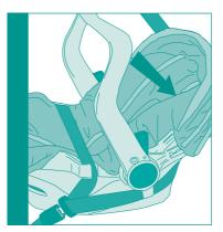
When fitted, the security of the child seat can be tested by pressing firmly into the backrest as shown.
