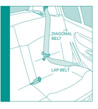
Your Mothercare child seat can only be installed rearward facing using a 3 point static or retractor seat belt, approved to UN/ECE Regulation No.16, or other equivalent standard.
