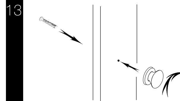
Use the supplied bolts to attach the knobs to the doors. Do not over tighten.
