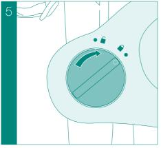
Secure this side of the tray in place by rotating the knob to the locked position, indicated by a locked padlock symbol.
