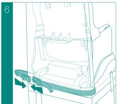
To avoid damage to the chair or buckle, both ends of the rear securing strap are adjustable so the buckle position can be positioned away from the corners of the chair.
