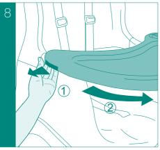
To release the tray, pull clip 1 outwards and swing the tray out, 2.
