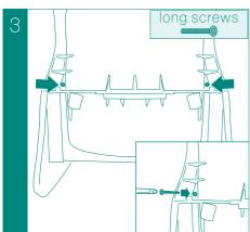
At the back of the seat, fit the two long screws where shown.
