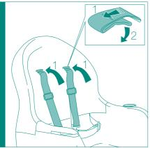
Push the ends of the shoulder straps through the backrest slots (1), and open the webbing out (2) so it cannot pull back through the slots.
