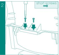
At the back of the seat, fit the two short screws where shown, using a medium size Phillips screwdriver.
