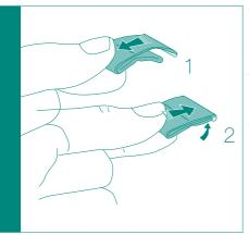
To remove the harness straps for washing, pinch the ends of the straps to flatten them, and pass them through the slots.
