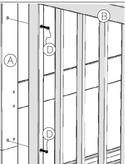
Use four bolts (D) to attach each fixed side (B) to cot ends (A). Do not fully tighten fittings at this stage.
