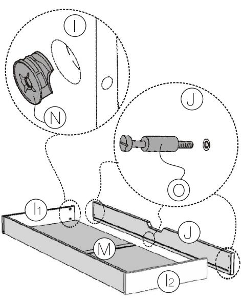
Screw 5 cam screws (O) into front panel (J). Insert 4 cam fasteners (R) into matching holes in sides panels (I). Align front panel (J) with base grooves to bottom. Then attach drawer front panel (J) to sides panels (I). Rotate cam fasteners (N) clockwise until secure, with a screwdriver.
