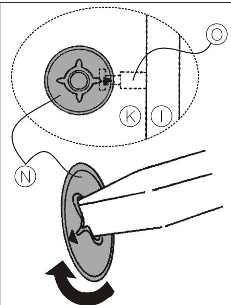
Ensure cam screws (O) locate in cam fasteners (N).
