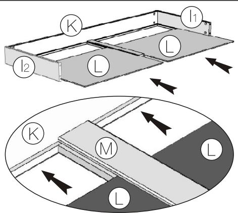
Slide in base panel (L) until it enters the groove in drawer back (K).
