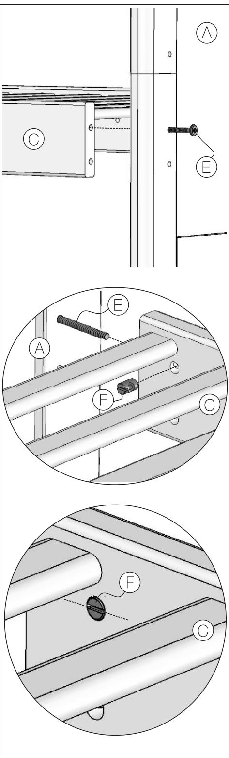
When assembling as a cot only use one barrel nut (F) on each corner of base (C).
