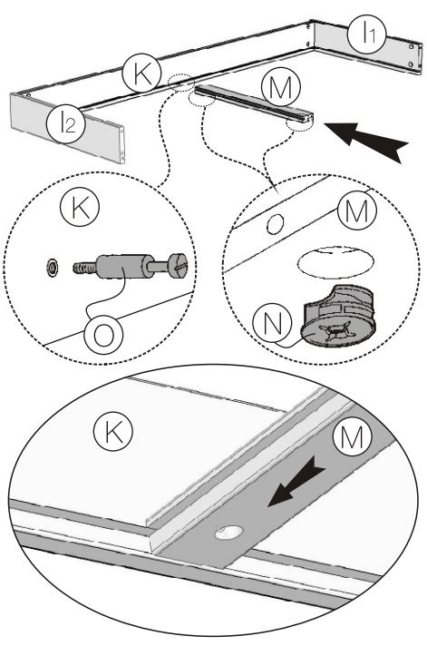
Screw 1 cam screw (O) into back panel (K).
