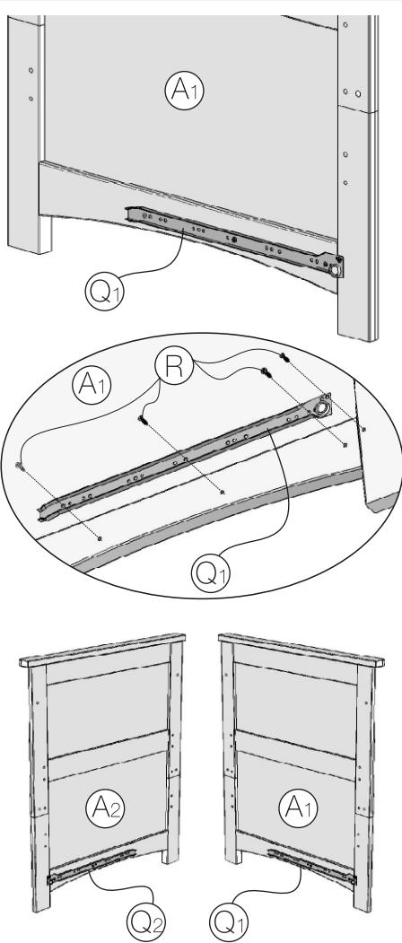
First fix metal runners (Q) onto bottom part of cot ends (A), with 4 small screws (R) in each metal runner.
