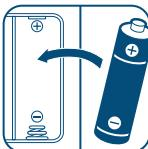
Take care to fit the batteries correctly observing the '+' and '-' sign marks on the battery and appliance.
