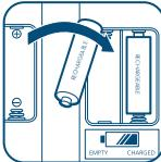
Rechargeable batteries are to be removed from the product before being charged (if removable). Rechargeable batteries should only be charged under adult supervision.
